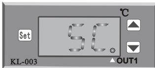
Press and hold the **Set** key to enter the menu, press the **Set** key twice to display **SC**, and then press the **▲** or **▼** key to correct the displayed temperature.
