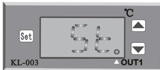
Press and hold the **Set** key to enter the menu, press the **Set** key three times to display **St**, and then press the **▲** or **▼** key to reset the parameters of the startup delay time.
