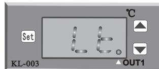
Long press the **Set** key to enter the menu, press the **Set** key five times to display **Lt**, and then press the **▲** or **▼** key to reset the lower limit parameter.
