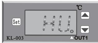
Press and hold **Set** key to enter the menu, press **Set** key again to display **HU**, and then press **▲** or **▼** to reset the hysteresis temperature parameters.
