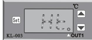
Press and hold the **Set** key to enter the menu, press the **Set** key four times to display **Ht**, and then press the **▲** or **▼** key to reset the upper limit parameters.
